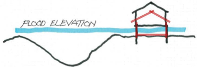
Figure 13: Graphic illustration elevation of structure.
